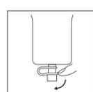
Remove the cap from the outlet tap and empty the pouch contents into the toilet or other approved container.
